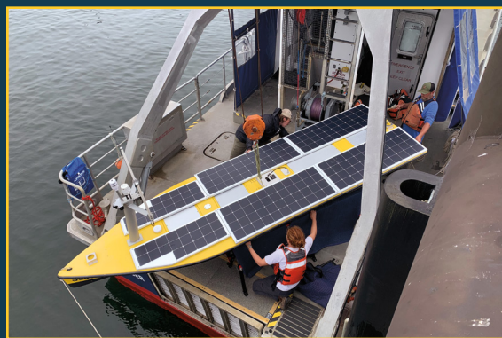
A new autonomous vessel equipped with sensors to detect harmful algal blooms. Photo: WHOI
